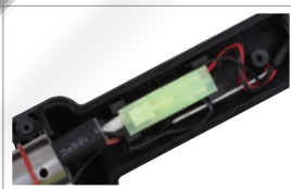
Quick change: Connectorized design for quick change heater
